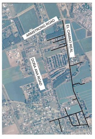
The Doña Ana MDWCA Phase I Southeast Collection system project includes base and bid alternatives that equal approximately 12,400 linear feet (LF) of vacuum sewer collection lines and related appurtenances on the following roadways/locations:
